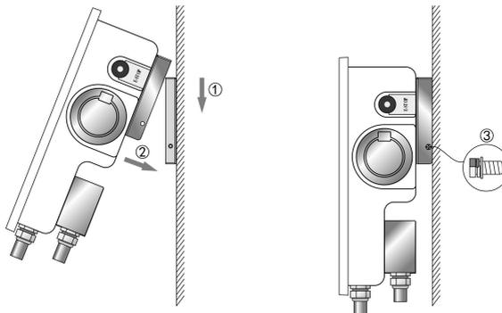
Fig. 5-7 Fix the wallbox on the wall
