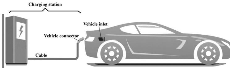
Fig. 3-2 Schematic diagram of CASE C connection
