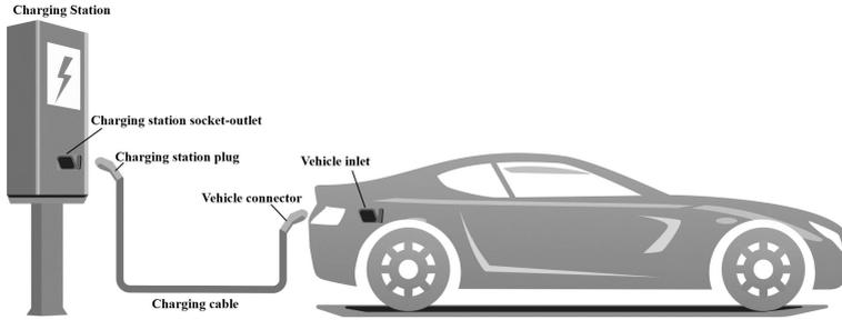
Fig. 3-1 Schematic diagram of CASE B connection
