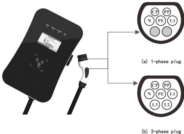
Fig. 3-5 Schematic diagram of Type 2 plug
