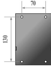
Fig. 5-3 Install the accessories on the wall
